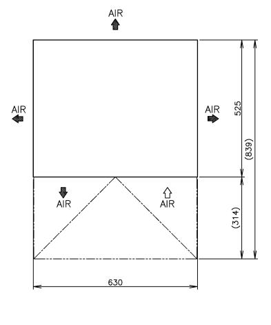
1. Install the ice maker properly in accordance with the instructions on location, water supply/drain connections and electrical connections stated in the instruction and installation manuals provided. Allow 10mm extra space at the installation site to meet any installation requirements (additional spacing is also required for proper air flow and pipe connections).
