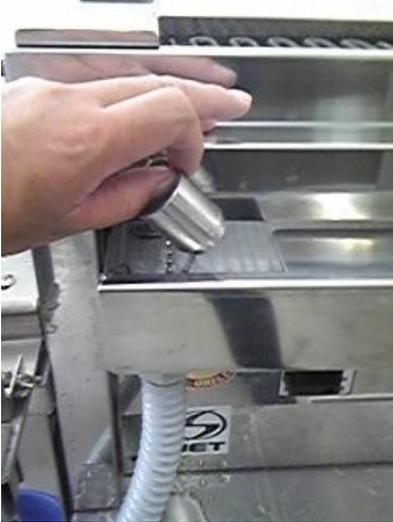
The drain hose is made of a PVC material and may become damaged if hot water is repeatedly made to flow through it. When draining water, be sure to first add cold water
