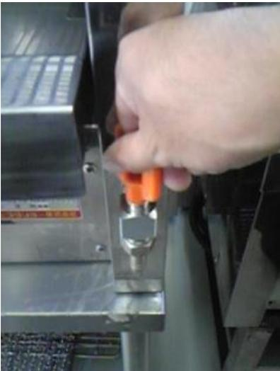
Turning the feed - water knob ( the orange - colored plastic part) too forcefully may damage it, so be sure to slowly when using it.
