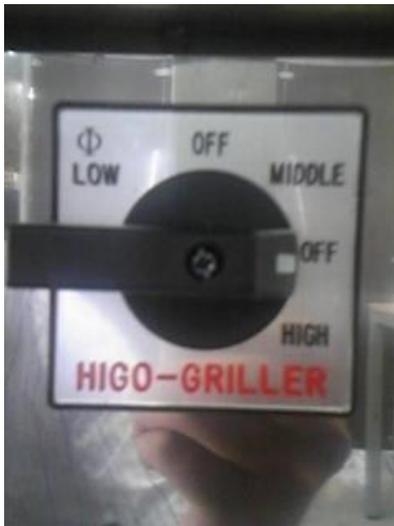
The switches each have three different settings( High,850°C (1562° F) , Medium, 600°C (1112° F); and Low, 450°C(842° F))
